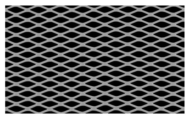
LW Aperture:14.22mmStrand Width:1.85mmSW Aperture:4.80mmThickness:0.90mmWeight:3.07 kg / m2Open Area:56%
